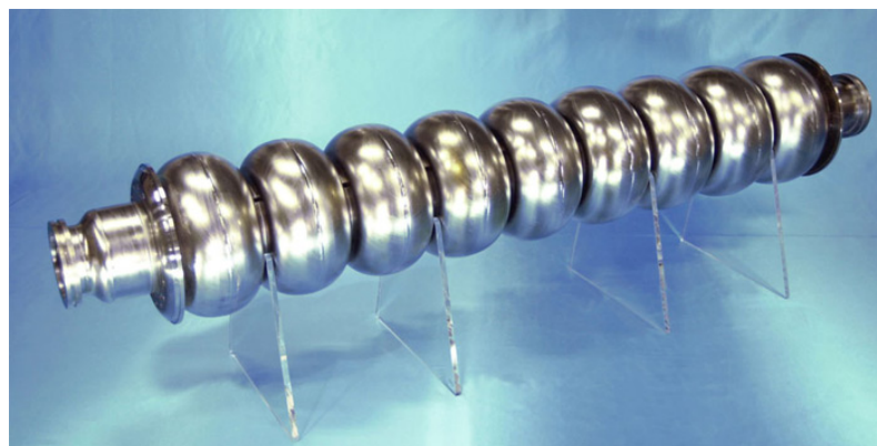
ILC prototype elliptical cell "p-cavity" (1.3 GHz): field alternates with each cell
