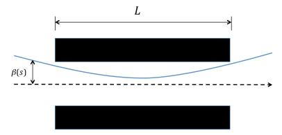
In this case, we clearly want to minimize the  $\beta$  function at the  $\mathit{ends}$  of the collimator.
