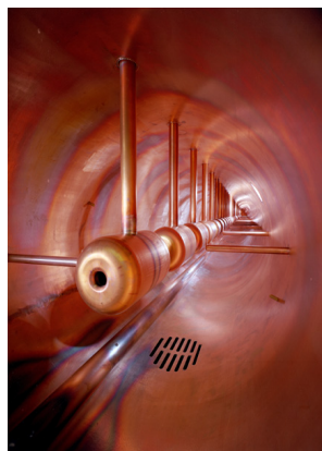
Fermilab Drift Tube Linac (200MHz): oscillating field uniform along length
