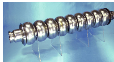
ILC prototype elliptical cell "π-cavity" (1.3 GHz): field alternates with each cell
