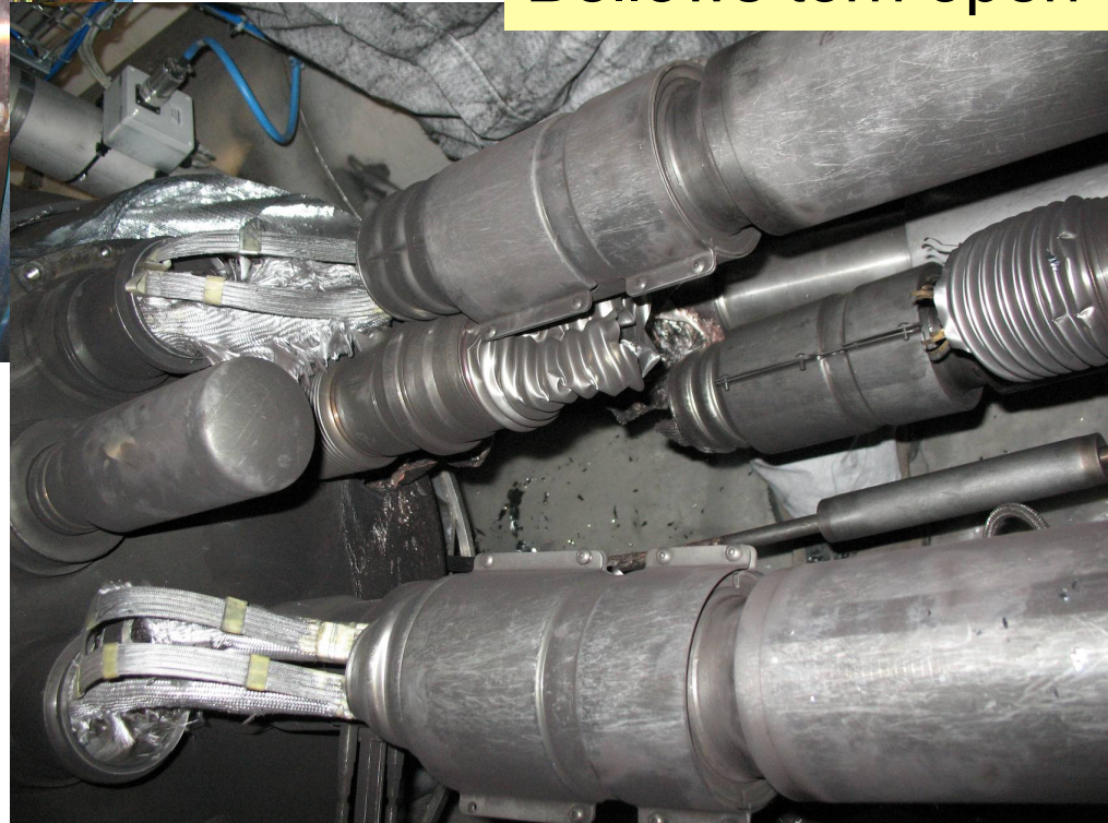
QBQI.27R3 Bellows torn open
