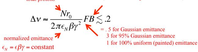
So the maximum injected charge grows rapidly with increasing energy
