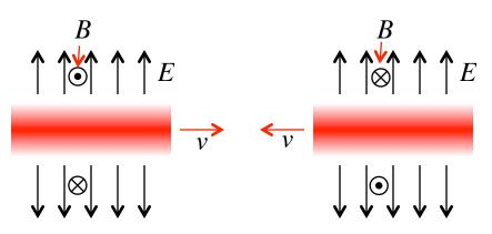
Both E and B fields are *repulsive* to the particles in the other bunch
