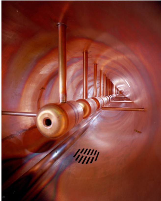
Fermilab Drift Tube Linac (200MHz): oscillating field uniform along length
