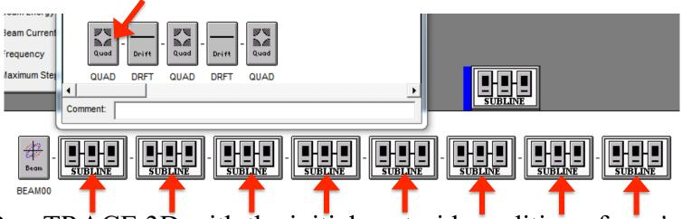
• Run TRACE 3D with the initial centroid condition of x=x'=0. Observe the orbit doesn't hold the 1 FODO cell period.
