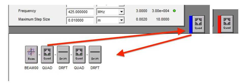
• The copy and paste works also for multiple elements. Let's make a beam line with several FODO cells.
